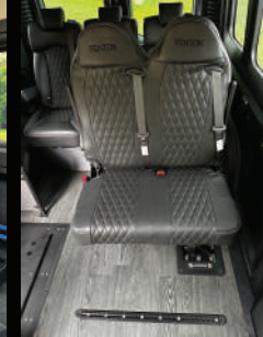
Double Bellagio Foldaway Seats with Fenton Mounting Plate and Black L Track
