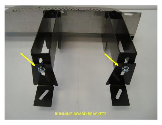
From the underside of the van mark the center of the angled slots to be drilled 9/16". Install the supplied 3/8-16" Rivet Nuts and Hex Head Flange bolts.
