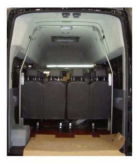
**Step 8** – Temporarily attach the Left and Right Horizontal Support Tubes to the main frame hoop and rear door opening anchor points. This will help establish the position of the mounting feet.
