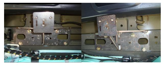
**Step 3** – Temporarily clamp the brackets in place and mark the hole locations. Remove the brackets and drill 4, 13/32" Dia. Holes for each bracket. Reinstall the brackets using 3/8" Hardware and re-secure and protect all wiring.
