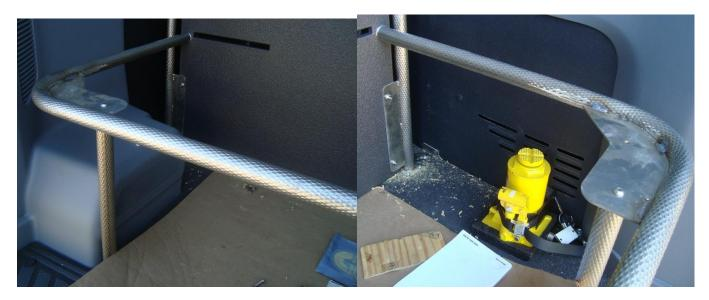
**Step 2** – Bolt the ends of the shelf perimeter tube to the lower partition panel using the 5/16"-18 Hex Head Bolts. These bolts are installed by reaching around the back side of the partition vertical tubes.
