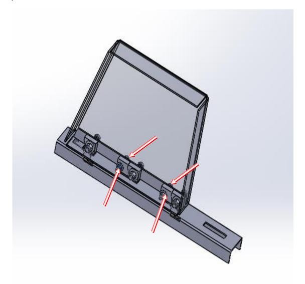
**CAUTION** – Seats MUST ALWAYS be locked into the AbiliTrax tracks and the Lock Hooks MUST ALWAYS be in the LOCKED POSITION and bolted in when a seat is in a vehicle. NEVER move a vehicle with a loose seat. NEVER attempt to occupy a seat which is NOT fully installed AND LOCKED in position. Occupied seats MUST ALWAYS be in the FORWARD FACING POSITION.
