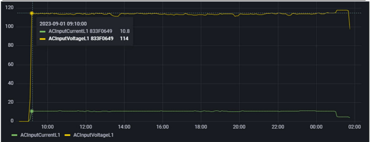
Figure3 – Actual Charging Voltage & Current
