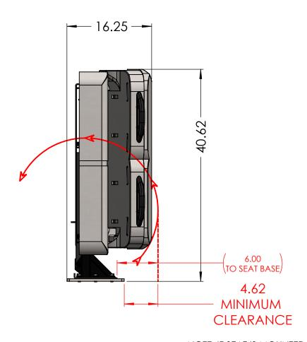
NOTE: IF SEAT IS MOUNTED LESS THAN THE MINIMUM CLEARANCE DISTANCE IT CAN RESULT IN DAMAGE TO THE SEAT FABRIC
